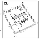
twist the wires from A back to the Fence Transmitter. See the "Install the Boundary Wire" section for more information on attaching the wire to a fence.
